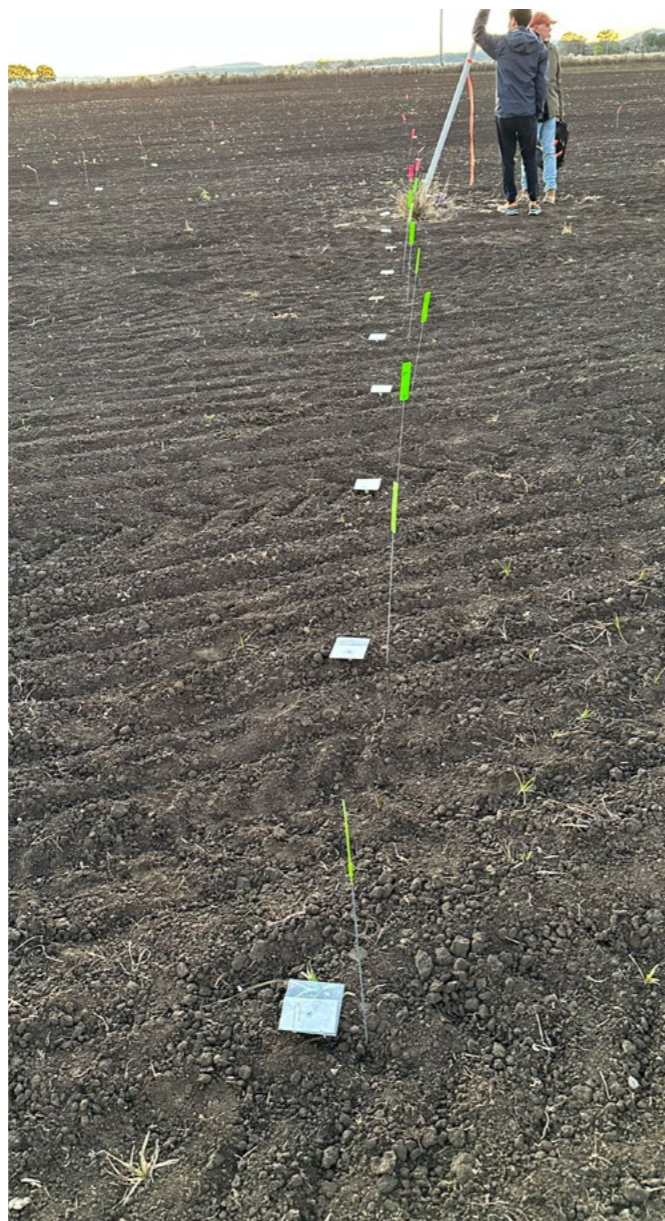
Ground droplet collection device
